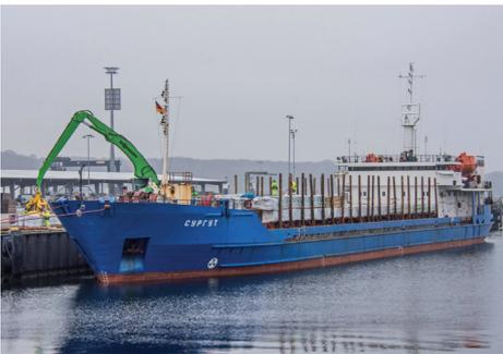
The load of one vessel is normally unloaded within two days by the colleagues of the SEEHAFEN KIEL Stevedoring using a gripper. The timber is then stored in the different port warehouses until it is finally delivered by road most of the time, however, the share of rail transport is growing.
